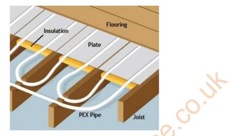
Specifically designed to sit between standard joists to hold pipes and spread the heat in a joisted floor installation.
