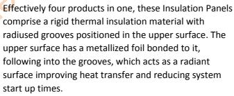
The grooves in the insulation securely retain our 12mm Pex-Al-Pex pipe in the correct position, eliminating the need for supplementary fixings.
