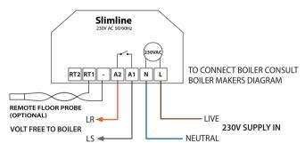
LS & LR ARE NORMALLY THE ROOM THERMOSTAT CONNECTIONS
