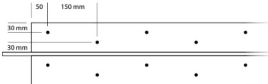
NOTE! Screw the plates after laying the pipes.
