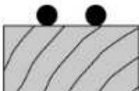
The grooves and joints of the boards must be glued using Casco mounting glue 3303 or the equivalent. The amount of glue must be generous so that an excess will be pressed out during laying; excess should then be wiped off. The amount of glue required is approx. 1.2 L per 10 square metres of floor area.
