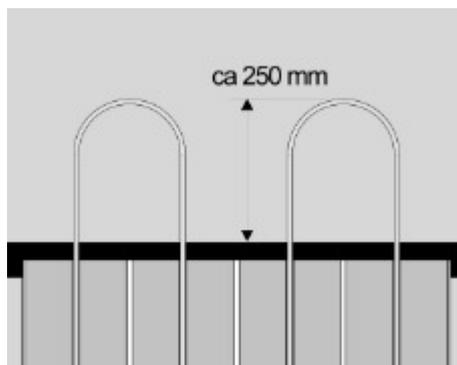
Press or tread down the underfloor heating pipe into the slot of the plate. After assembly the pipe must lie in the slot and must never under any circumstances touch the over-lying floor.
