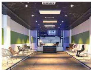
Ceiling mounted U+ infrared heating panels
